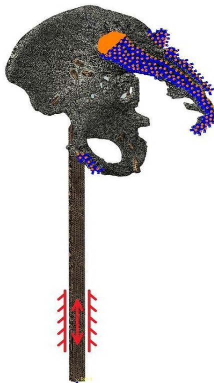
Fig. 6. Boundary conditions imposed on the model
