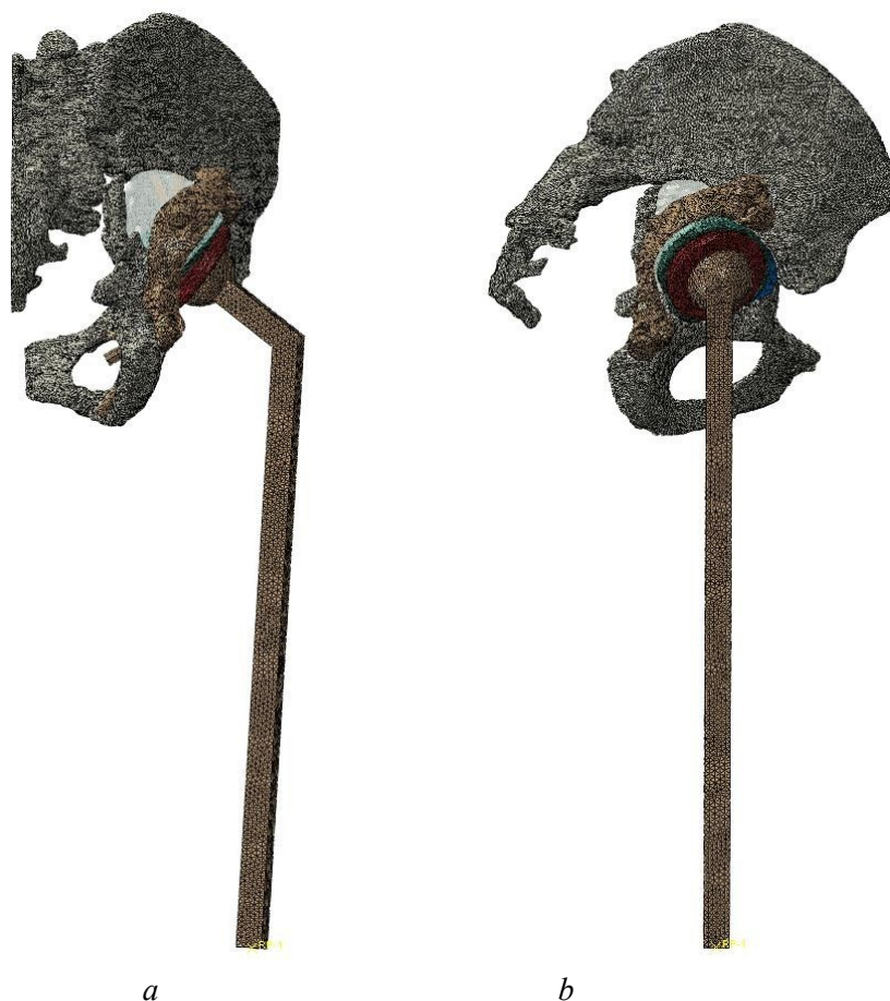
Fig. 5. Computational model of the skeleton-prosthesis biomechanical system: front view ( a ), right view ( b )
